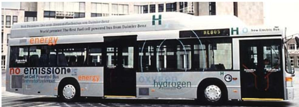
Figure 4 FC bus by Daimler: the NEBUS
