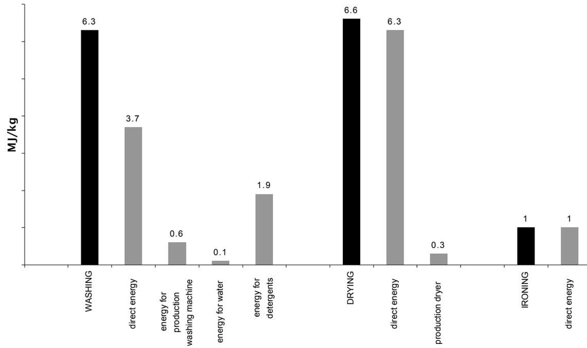
Fig. 6 Direct and indirect energy requirements for domestic washing, drying and ironing (MJ/kg)
