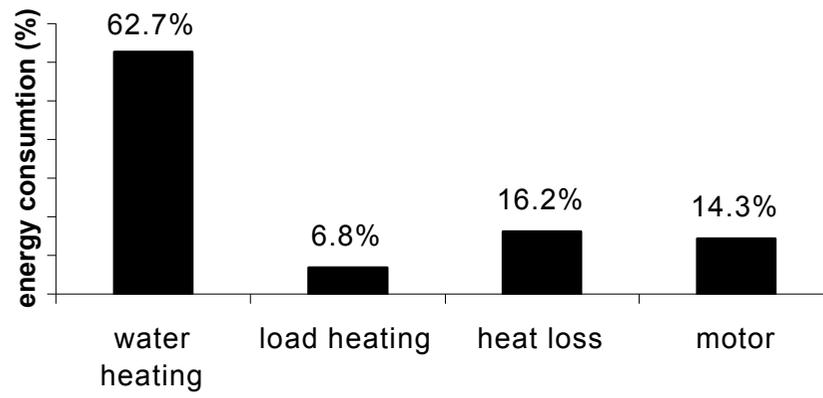
Fig. 7 Energy consumption breakdown for an average washing machine in Europe (60° C cotton cycle)
