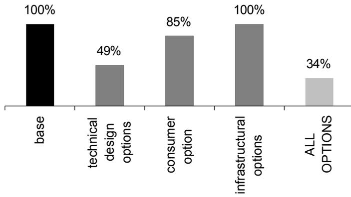
*Fig. 12 Washing machine water savings potentials: technical design, consumer and infrastructural options*
