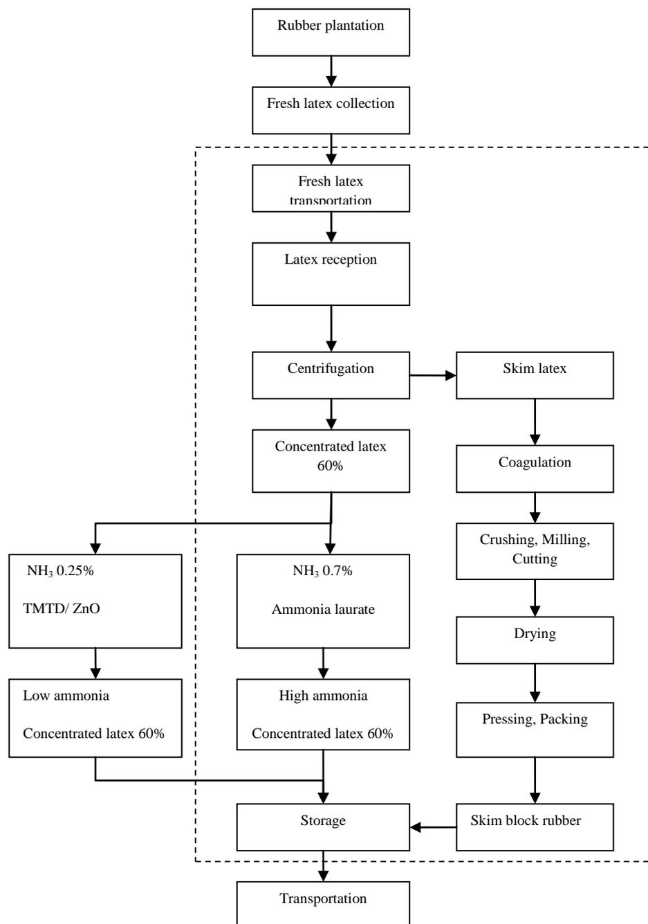
**Figure 1** Schematic diagram of concentrated latex production. The dotted lines indicate the system boundary of this study. See text for explanation.
