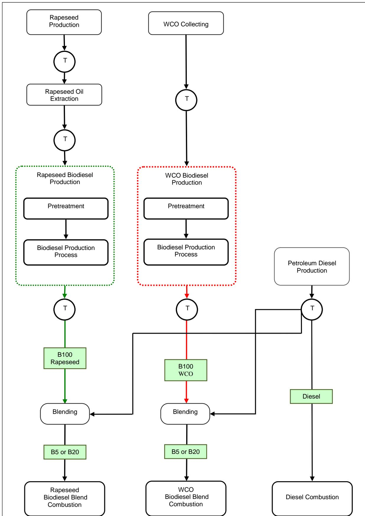
**Figure 1. System boundaries for biodiesel and diesel utilization included in the study (T: Transport)**
