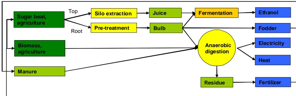
The concept illustrated above includes a decentralised silo storage system for the sugar beet top. The root is pre-treated at two stations. The root is first cut into small pieces and afterwards pressed. The juice which is rich in sugar can then be fermented into ethanol in a low cost 1. generation system that renders the use of expensive enzymatic treatment obsolete. The residue from the bulb can subsequently be used as animal feed or as input for the biogas plant.
