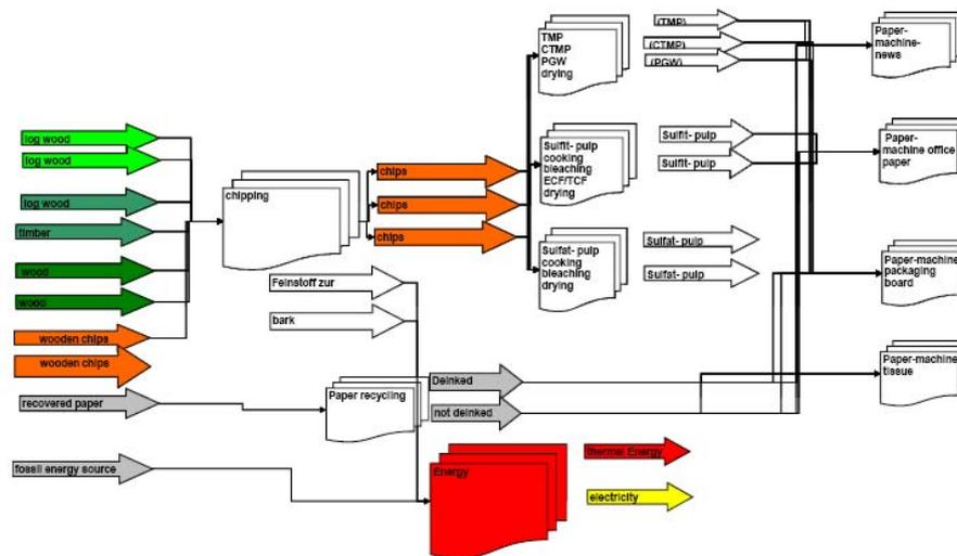
Figure 2: flows and aggregated processes in the paper production system
