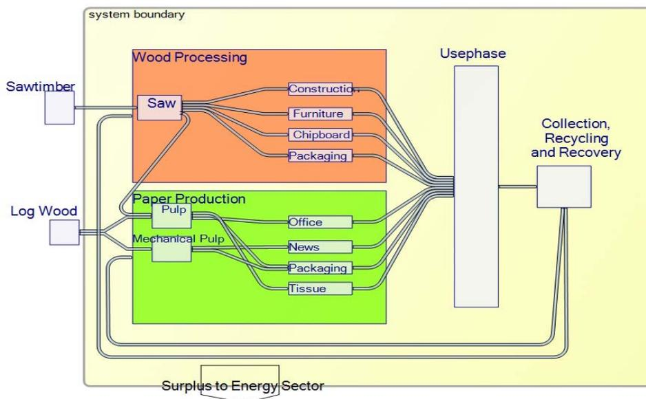
Figure 1: System boundary, main material flows, main processes
