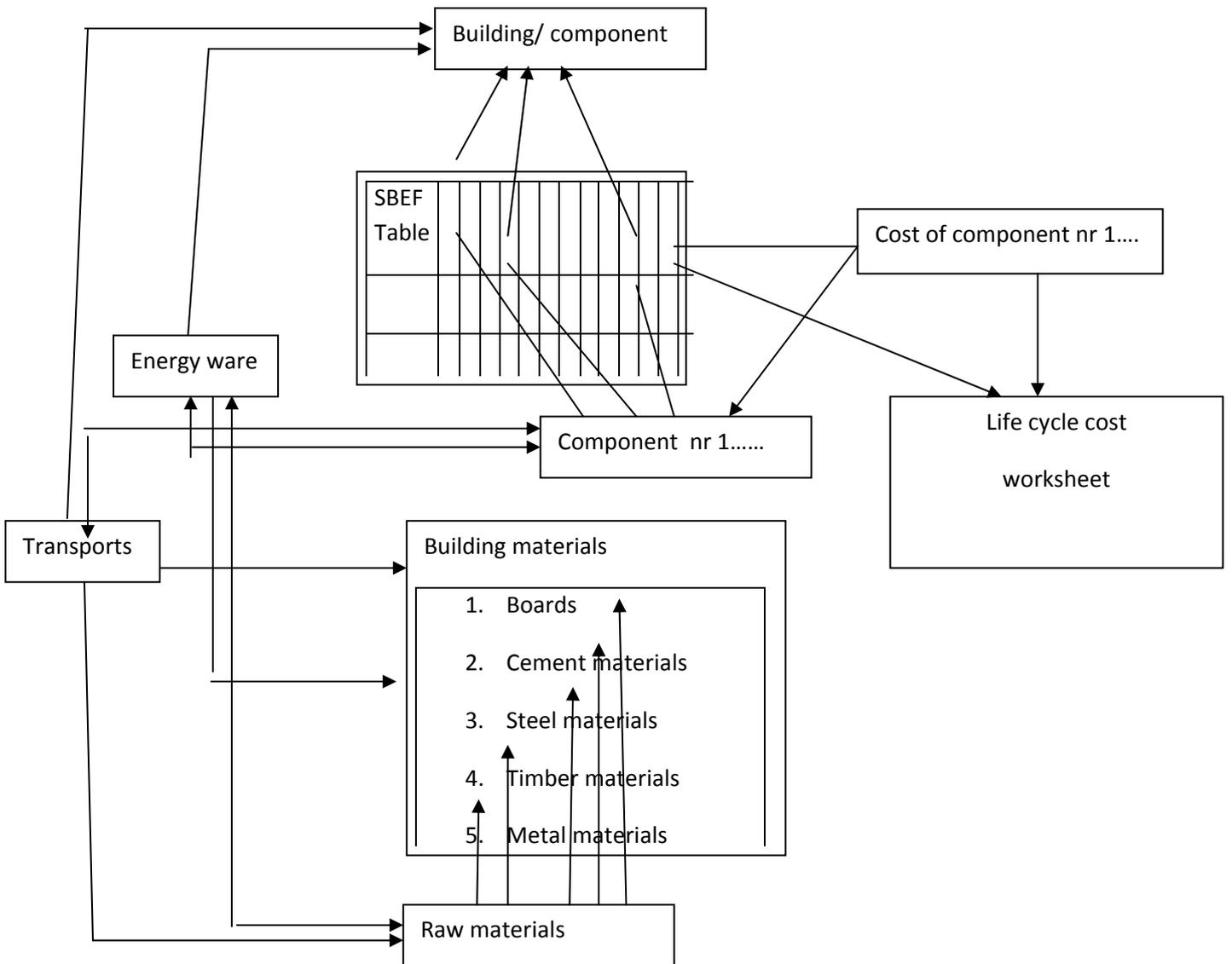
Figure 23 the complete data structure that organizes the inventory data for the first inventory phase for life cycle assessment of building
