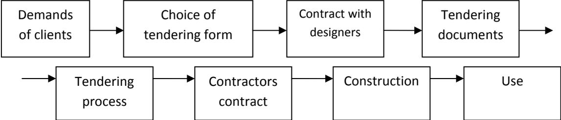
Figure 9 Design and Construction process
