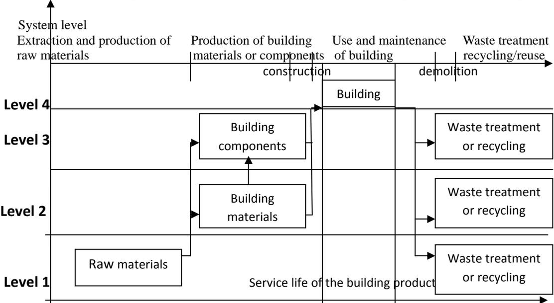
Figure 6 System levels in a building products life cycle (Jacbo 2001)
