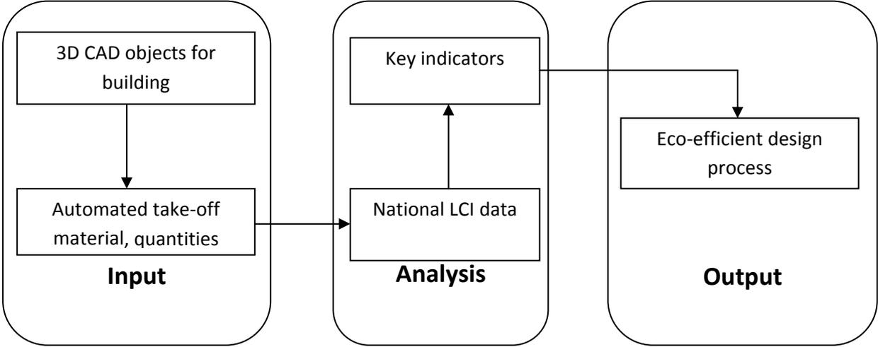
Figure 7 Essential steps for 3D CAD modeling and environmental evaluation tool (Seo 2003)
