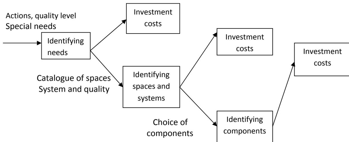
Figure 12 LCC on different stages of building design (Paulakka 1999)
